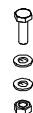
Fixings M8 x 30 Hex head screw, nut & washers, common to all steelwork joints
